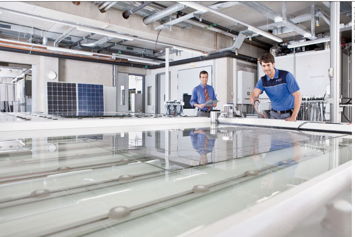
In one of the tests, the module is submerged in a water bath at 22 degrees Celsius.
