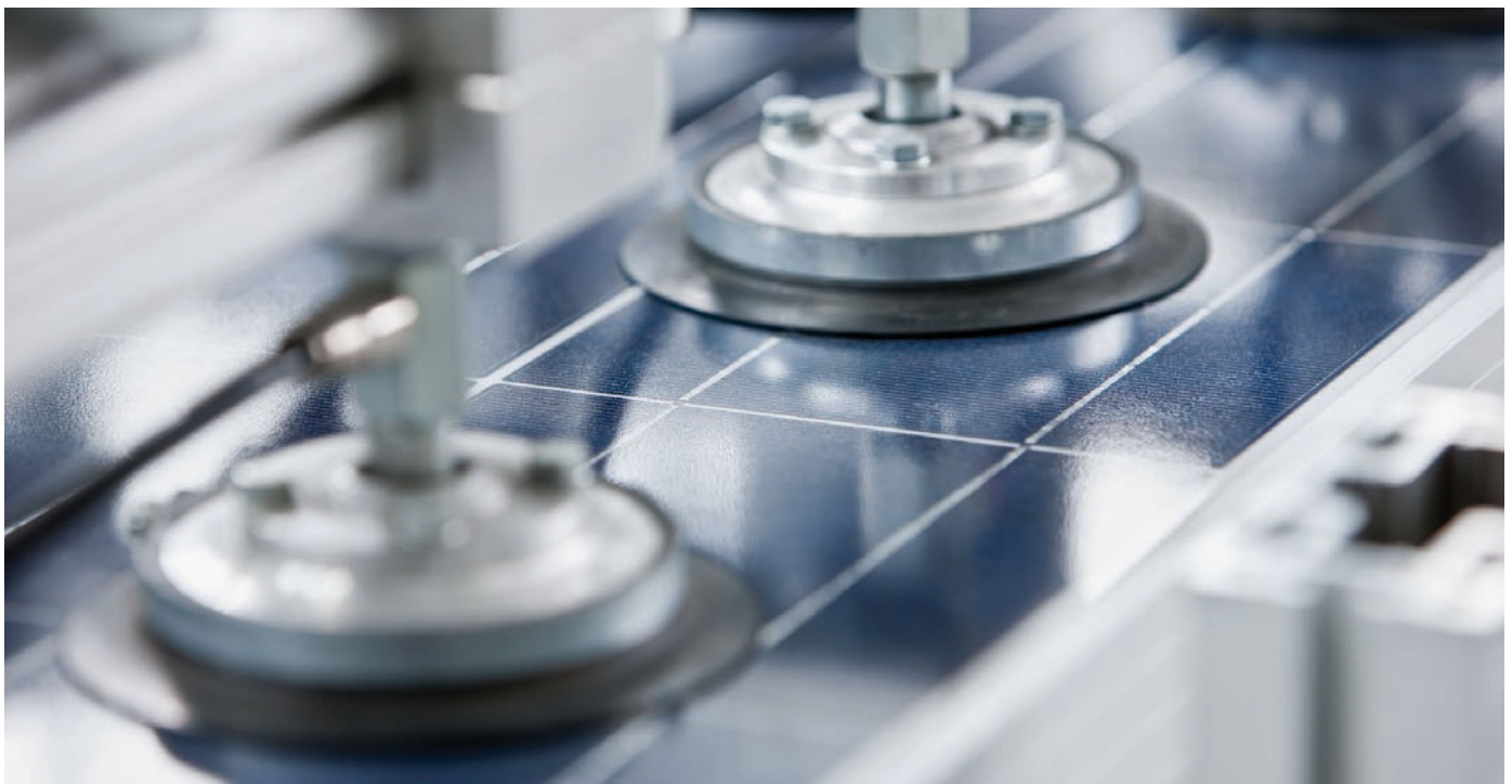
The module later undergoes a mechanical load test, which simulates snow and wind loads.
