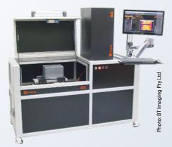
The cetisPV system utilizes xenon light source technology, with a lamp lifetime of up to three million flashes, dependent on the parameters.
