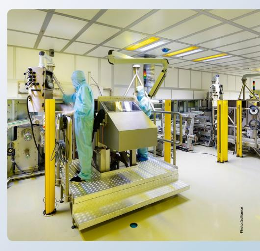
coating line developed by Solliance is for both perovskite and electron transport layers. Using a commercially available PET/ITO foil, coating, drying, and annealing processes were executed under ambient conditions at a rate of five meters/minute.
