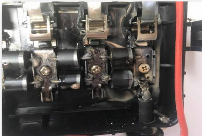
Panel Diode Failure
