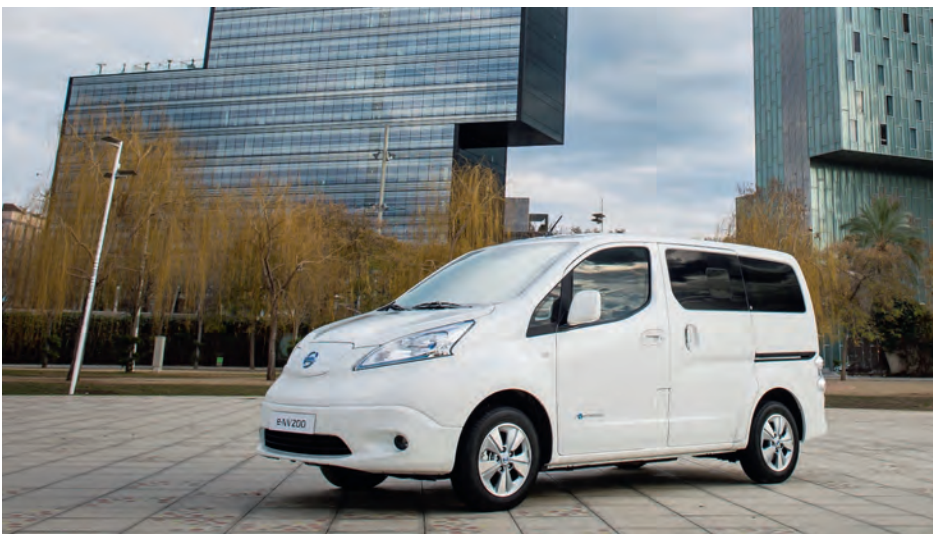
The 2018 Nissan e-NV200 features a 40 kWh battery. Nissan is one of a few companies that have already begun to roll out vehicle to grid technology, although so far only in certain markets, in a limited capacity.
