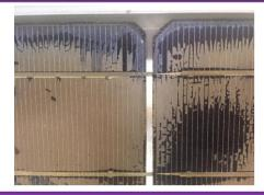
Busbar corrosion, delamination, and EVA browning in JRC glass-glass module study
