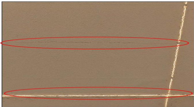
Cracks extend the length of the module across busbars
