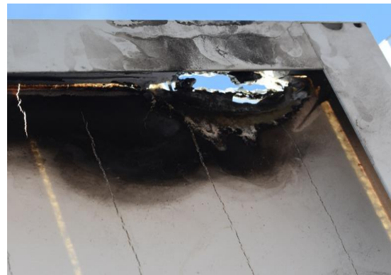
Overheating leading to burning
