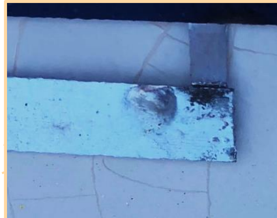
Cracking leading to corrosion
