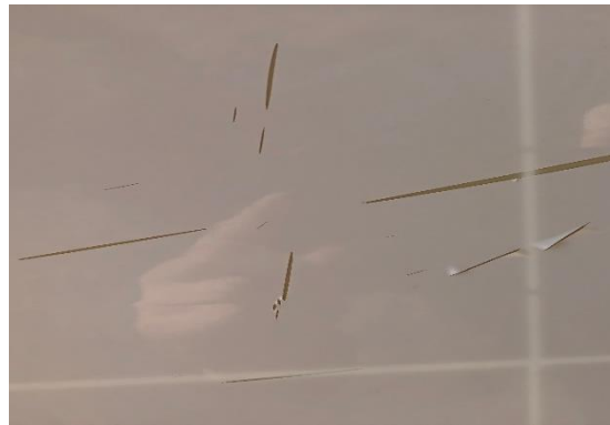
widespread cracking of backsheet outer layer
