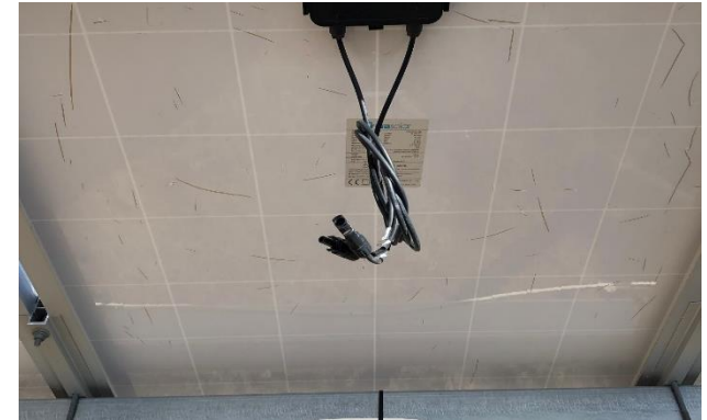
widespread cracking of backsheet outer layer
