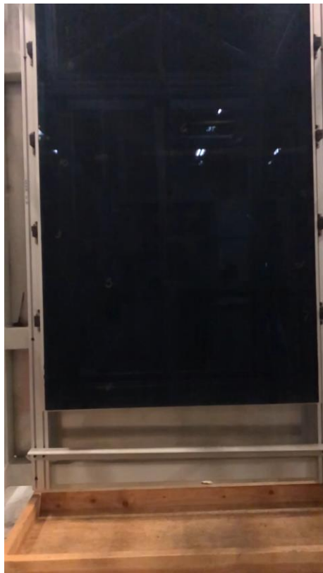
First Solar S4 Test Oct 2019 (pictured) and S6 Test Jan 2020 per IEC 61215-2 MQT 10.17 75mm diameter hail
