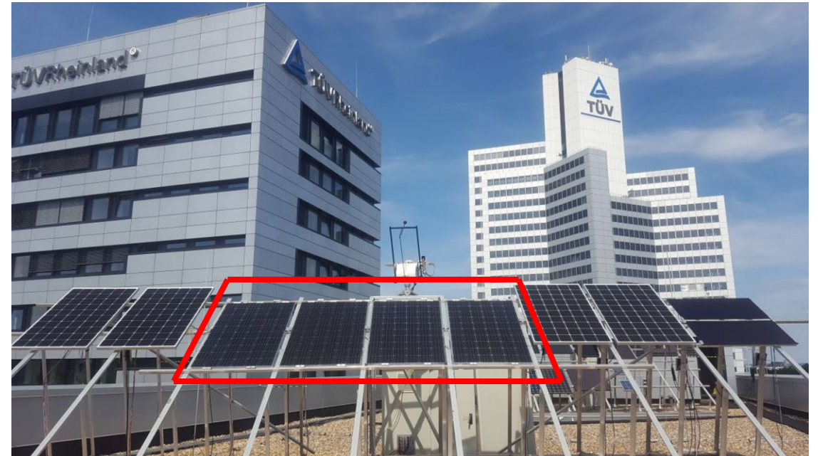
Mounting rack with mono-facial, bifacial (Height above ground = 1.5 m) , and thin-film PV modules
