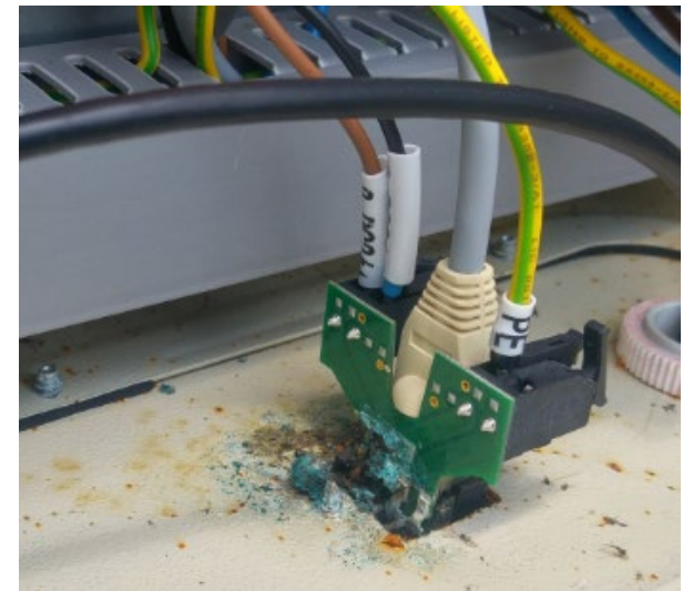
Water leakage through cable gland
