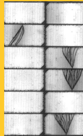
Cracks propagate post MLT
