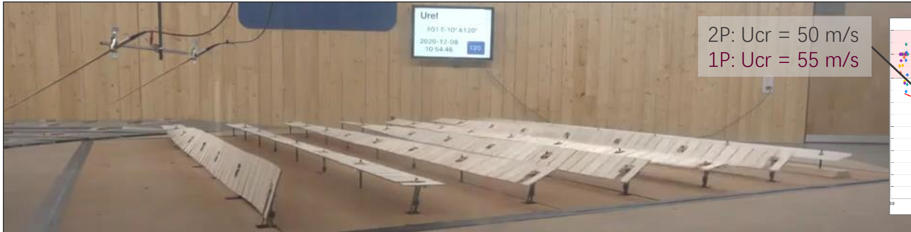
Traditional Tracker - Wind Stow at 30 Deg
