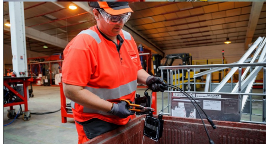
Aluminum frame, junction box, and cables are removed and recycled.
