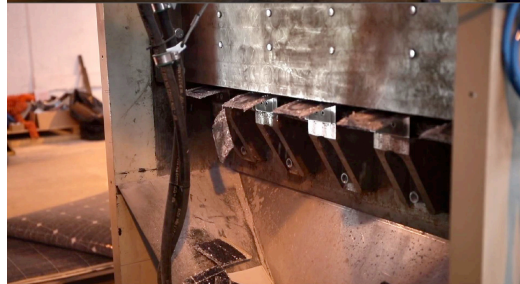
The laminate is cut into slice with fixed size.
