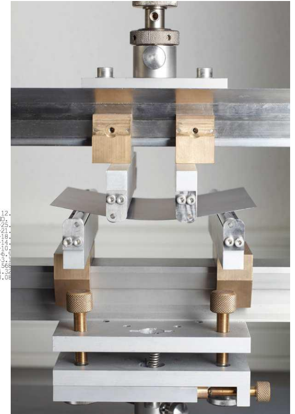
4-point-bending (mc-Si Wafer)
