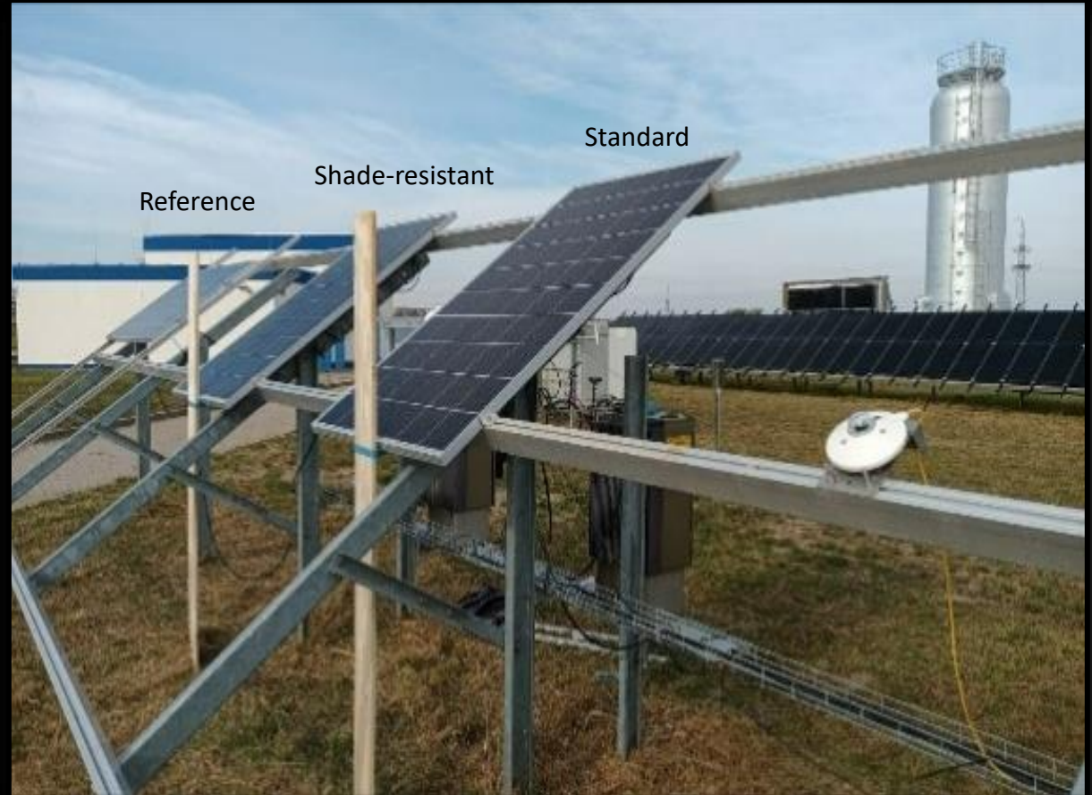
Energy yield measurement setup at the Anhalt Photovoltaic Performance and Lifetime Laboratory (APOLLO) in Bernburg, Germany
