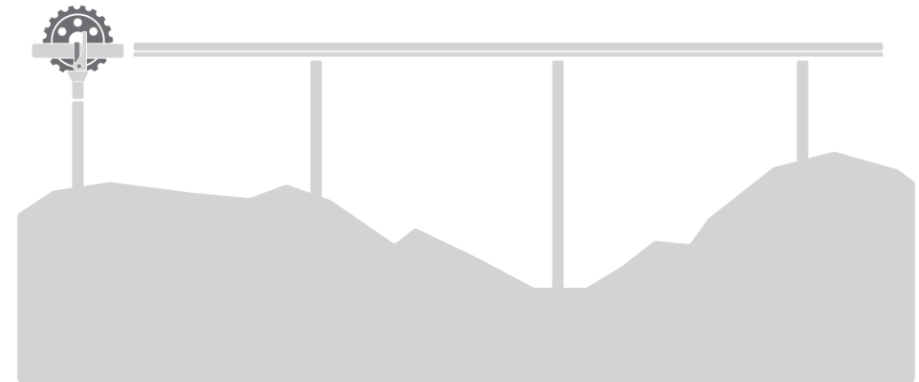
Continuous Torque Tube Tracker on terrain with variable piles
