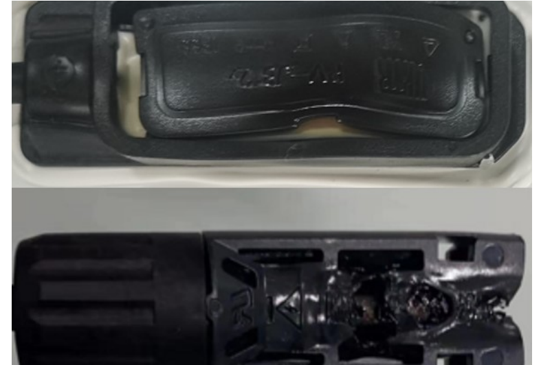
Junction box melt after thermal cycling
