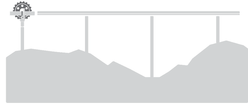
Continuous Torque Tube Tracker on terrain with variable piles
