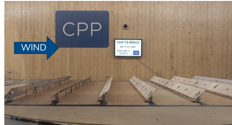
At high tilts: minimal deflection + less motion
