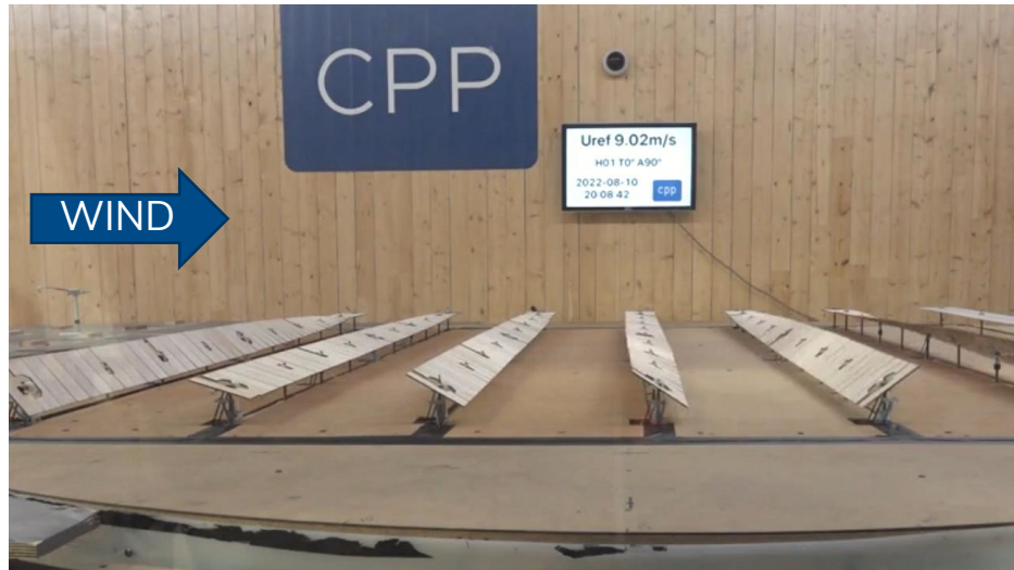
At low tilts: significant deflection + angular motion
