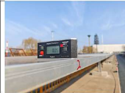
Fig.5: Target rotation angle 0°, non-driven 1 component angle
