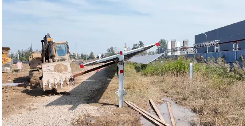
Figures: Snapshot of pluck tests on the ESET system (middle) and heaving mode shapes (right)
