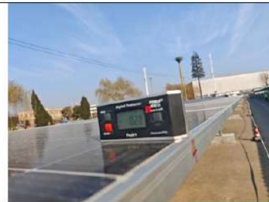
Fig 7: Target rotation angle 0°, non-driven 3 component angle
