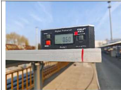
Fig.4: Target rotation angle 0°, south end component angle
