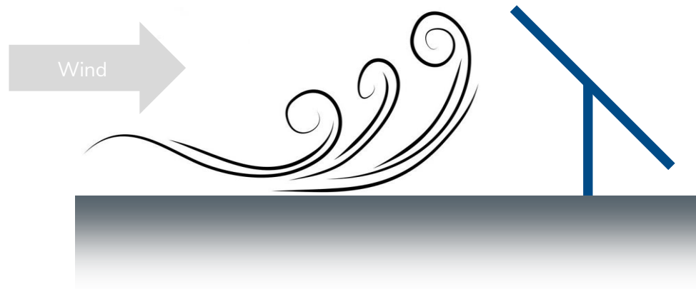
Figures: Peak pressure locations on the system in uplift
