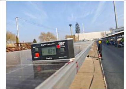
Fig 6: Target rotation angle 0°, non-driven 2 component angle
