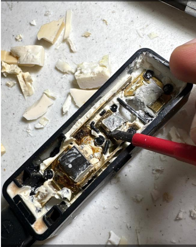
Teardown: ribbon not bonded to the contact pad
